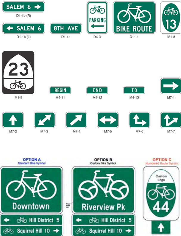
Figure 9B-4. Guide Signs for Bicycle Facilities
